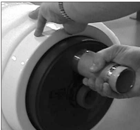
Fig. 2.1.15 - Installing head assembly by hand
