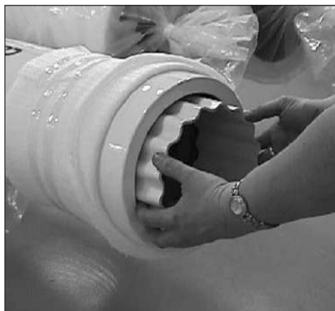
Fig. 2.1.13 - Installing Thrust Ring
