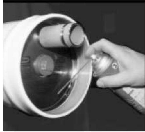
Fig. 2.1.6 - Applying penetrating fluid
