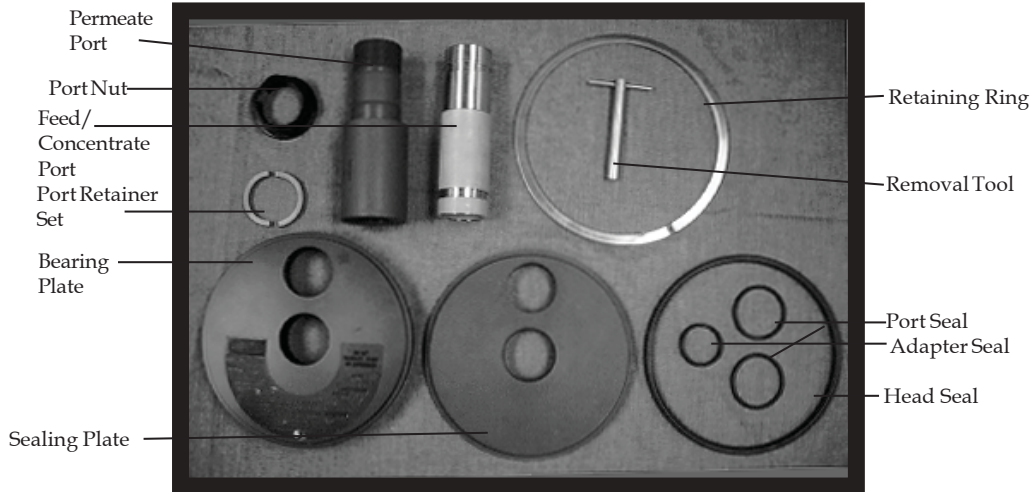
Fig. 2.1.4 - Head component identification - head disassembled
